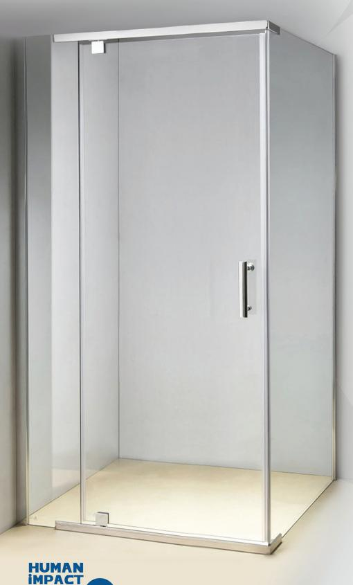
Frameless shower doors or panels must be glazed with Grade A toughened or toughened laminated safety glass with a minimum thickness of 6 mm, in accordance with AS 1288
