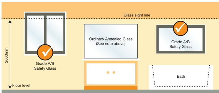
Ordinary annealed glass may also be used behind a vanity unit providing the fixed vanity or bench has a height of not less than 760mm and a width of 300mm that extends to the full width of the glass or mirror.
